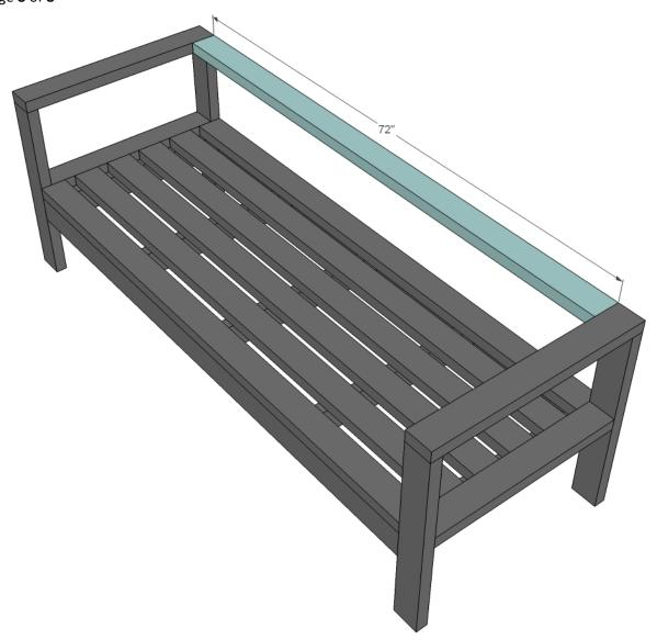
Finally, attach the back. This time, use 2-1/2" pocket hole screws.
