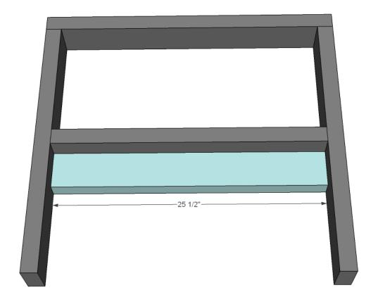
To finish the arms, add another board underneath. We'll use this board to tie into the seat framing in the next step.
