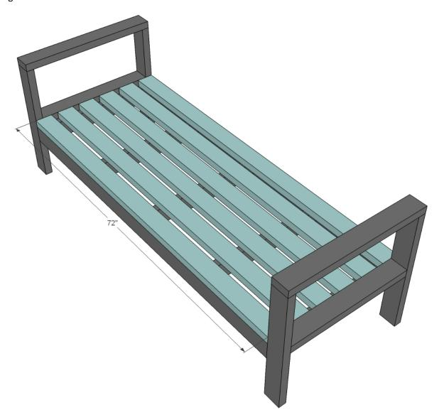
Now we can start adding the seat slats. Just screw down to the seat framing with 2-1/2" exterior decking screws.
