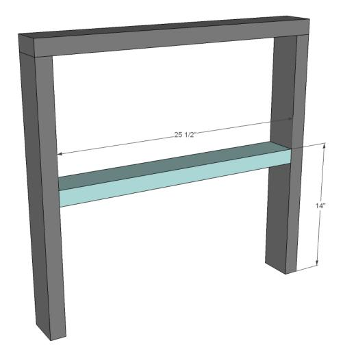
Next, add the supports, 14" up from the bottom of the legs with 2-1/2" decking screws.
