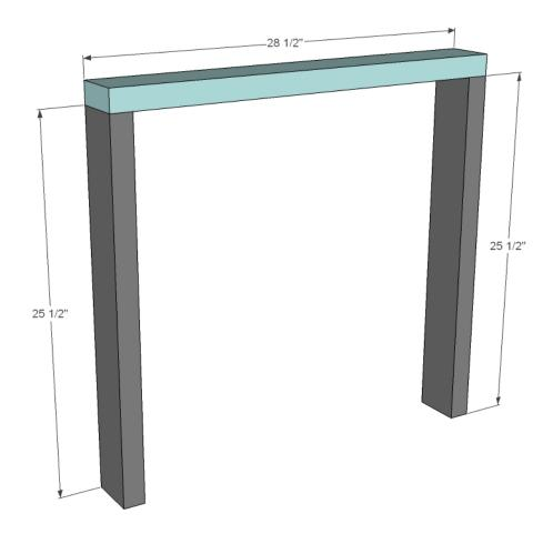
We'll start the arms by attaching the armrest to the two legs. I'm using 2-1/2 exterior decking screws.
