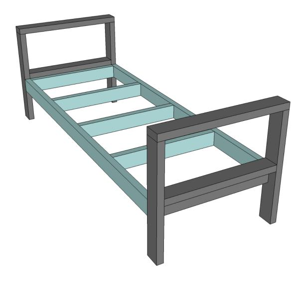
Attach the seat framing to the arms with 2-1/2" exterior screws.
