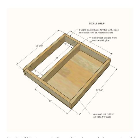
Step 2: Build the two smaller frames, but only cover the larger portion of the tray bottom in plywood.
