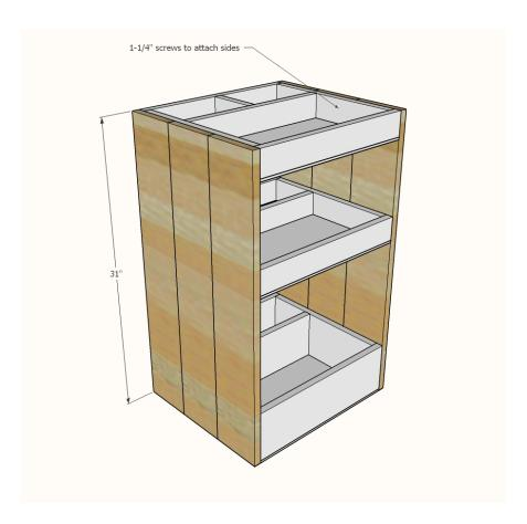
Step 4: Attach the sides to the three trays. I attached the outer 1x6 boards first, and then centered the remaining middle 1x6 leaving small gaps in between.
