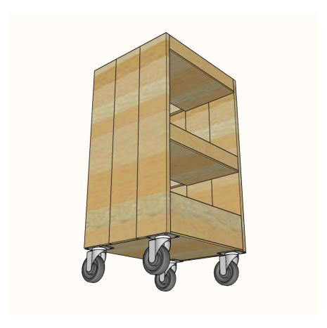
Step 6: Attach caster wheels to base of project with screws.
