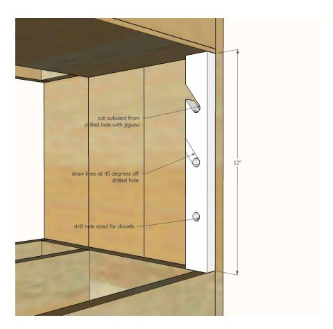
Step 5: The ribbon holder is easy to make. Just drill holes in a 1x3 board in the center where you'd like your ribbon dowels to be placed. Then, starting from the hole, cut outward with a jigsaw to create a channel for the dowels to slide in. Attach the 1x3 to the inside of the project with 1-1/4" screws (so it can be removed too).
