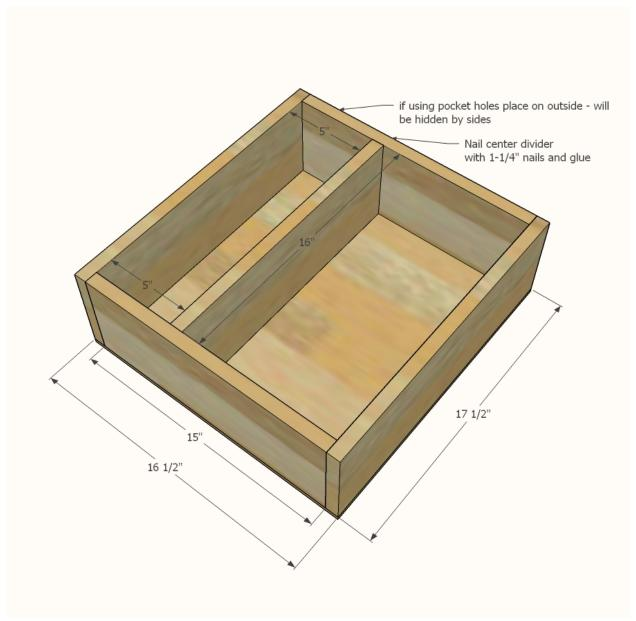
Step 1: Build the bottom tray. 1x6s can be attached with 1-1/4" pocket hole screws or 2" self tapping screws. The divider can be nailed or screwed in place. Attach bottom plywood with glue and  $\frac{3}{4}$ " finish nails.
