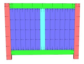
Frame the two larger panels with 2 x 4 pieces. All of the pocket holes in the 2 x 4's should be for 2-1/2" pocket hole screws except the pocket holes that will be used to secure the top. Those need to be drilled for 1-1/4" pocket hole screws. Assemble everything with glue and pocket hole screws. Make sure the panels are flush with the 2 x 4's on the side with the pocket holes.
