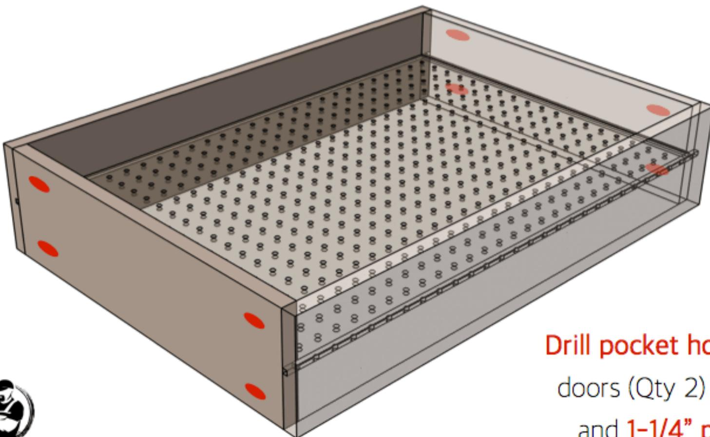
**Drill pocket holes** and assemble doors (Qty 2) using wood glue and  **$1-1/4''$  pocket screws.**
