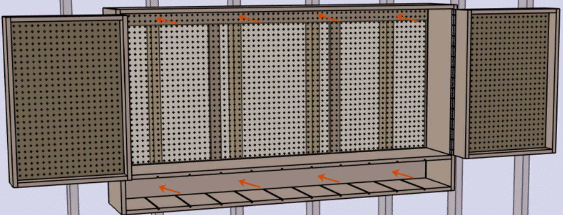
Locate studs, check for level and anchor wall unit with **2-1/2" wood screws**.
