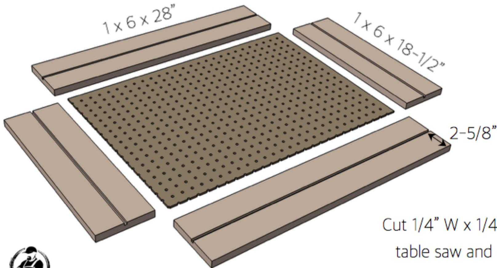
Cut  $1/4''$  W x  $1/4''$  D dados using table saw and dado blade or router and  $1/4''$  spiral downcut bit.
