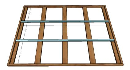
Step 4: Attach longer grid moulding pieces inside frame, to all back support boards, with 1-1/4" nails and glue. TIP: Use the 12" long moulding pieces as guides.
