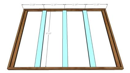
Step 3: Attach back support pieces to back, nailing from outsides with 1-1/4" brad nails and glue.
