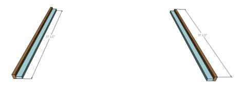
Step 1: Attach two of the 37-1/2" long 1x2s together in an L shape with 1-1/4" brad nails and glue. Build two.
