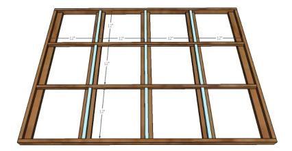
Step 5: Attach shorter grid pieces in between longer grid pieces with 1-1/4" nails and glue. Use the shorter grid pieces that you haven't attached yet as guides.
