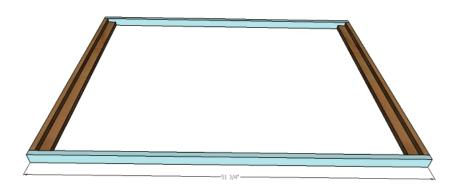
Step 2: Attach longer 1x2s to the project, outside edges flush, with 1-1/4" brad nails and glue.
